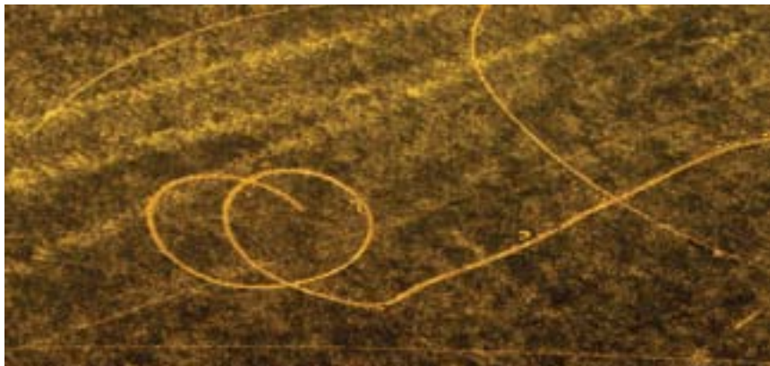
This aerial image depicts a textbook circular prop scar left by a skiff jumped on plane in water that was too shallow.
